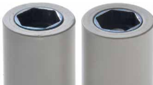
FIGURE 3 2-piece ISBs with a different height of the base due to incorrect assembly. Assuming that the right is the correct one, the use of the component on the left would lead to a vertical incongruity of the position of the analog and, subsequently, a possible under occlusion of the FDP
