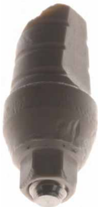
FIGURE 2 Wear of a PEEK ISB due to multiple uses
