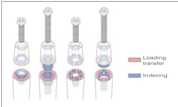
**Fig 4a** Force transmission versus indexing in flat-to-flat abutment connectors. In flat-to-flat configurations, the surfaces intended for force transmission are perpendicular to the clamping forces of the screw.
